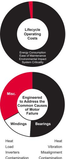
Contamination Contamination Voltage Issues Lubrication Issues Electrical Discharge Stress, Load, Fatigue
